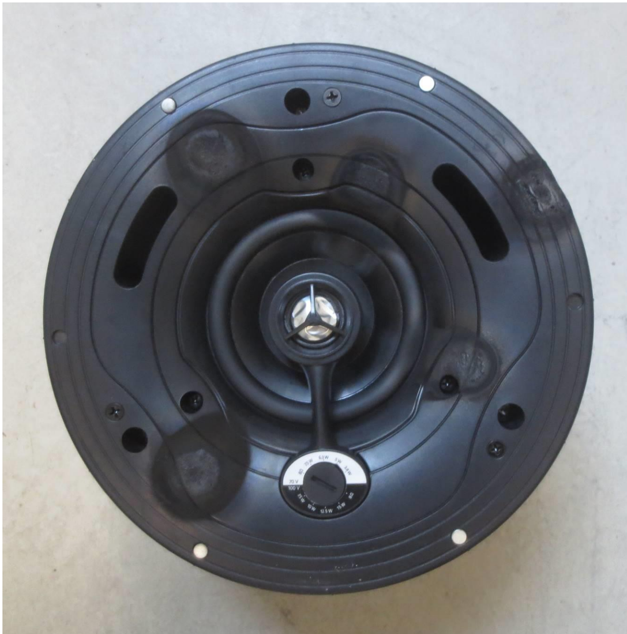
04 Test item after test, flame application points 01 to 04
